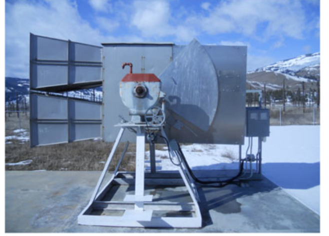
Figure 8. Calibration Horn system seen from the East. Two identical horns are mounted piggyback. The electronics is housed in the casing on the back of the horns. Antenna driving is manual, using the large declination scale for pointing. The upper horn is the one currently used.
