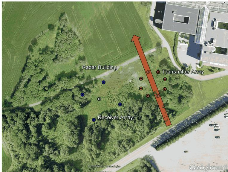
Figure 3.2: Overview picture of the setup of the SKiYMET radar at Dragvoll. Picture from [9]
