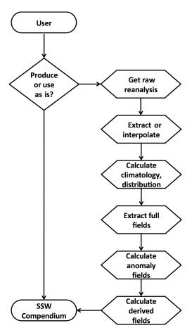
**Figure 2.** Flowchart showing how the SSWC can be used as is or the different steps to produce the dataset.
